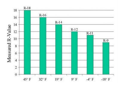
In full-scale attic tests at Oak Ridge national Laboratory, the R-value of 6 inches of cubed loose-fill attic insulation progressively fell as the attic air temperature dropped. At -18 F, the R-value measured only R-9. The problem seems to occur with any low-density, loose-fill fibrous insulation.
