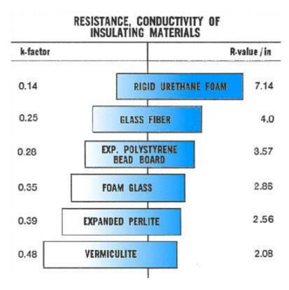
With the lowest k-factor and the highest R-value, urethane foam can provide more thermal resistance with less material than any other insulation.
